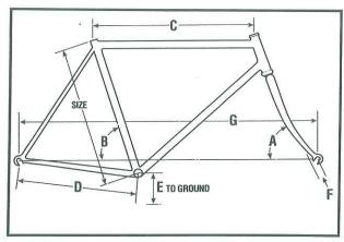
**Seat Tube Length (Size)** - The distance from the center of the bottom bracket to the top of the seat tube, although alternate methods may measure to the center of the top tube or top of the top tube. This relates to overall leg length, but with the advent of super-long seatposts and new frame designs like the Y bikes (which don't have a true seat tube), seat tube size is less meaningful than it once was.
